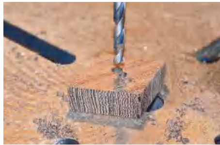
▲ Pic.14 I used the drill press to cut out three 10mm holes. Using small files, I enlarged these into the shape of the brass keyhole escutcheon
